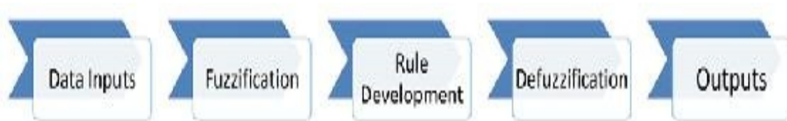
Figure 25. FIS functionality diagram. Note that the fuzzy representation of the data involved is in this form only within the system itself, as the outputs (prediction and rules) are always crisp.
